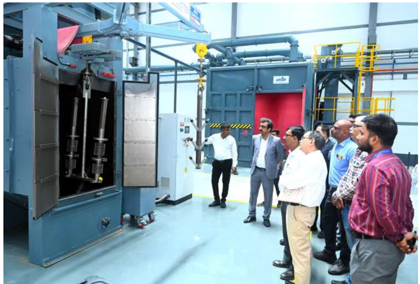
Wheel-blasting machines (hanger type): for efficient and rapid treatment of metallic parts
